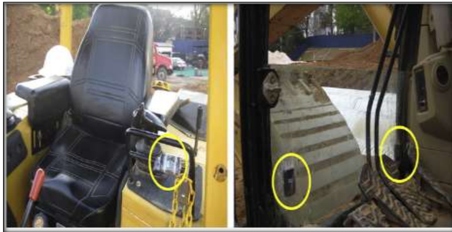
Fig 4: a) GPS Data Logger Mounted on a Loader b) Two Units Mounted Inside an Excavator Cabin
