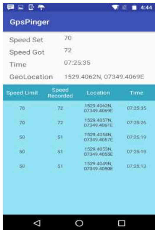
Fig. 7: Android Application Showing Real-time Data
