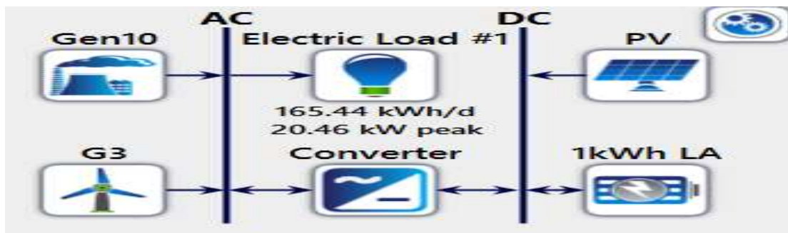
Fig. 5. Model of Hybrid Power System with Wind/PV/Generator
