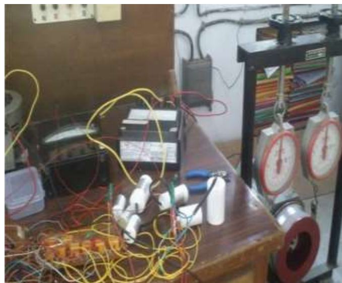
Fig. 7 Complete Assembly of Motor Along with APFC
