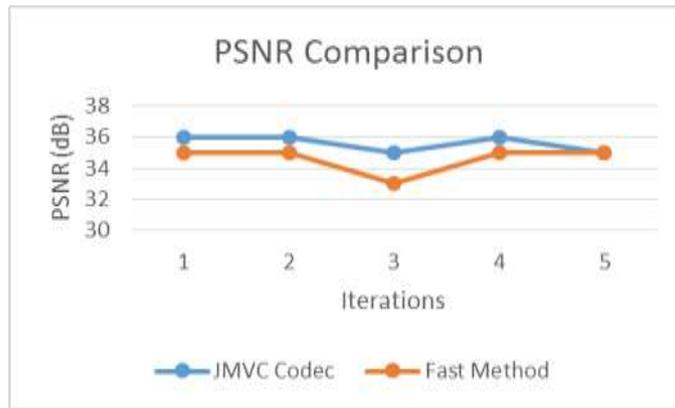
**Fig. 3. Ballroom Sequence PSNR Comparison**
