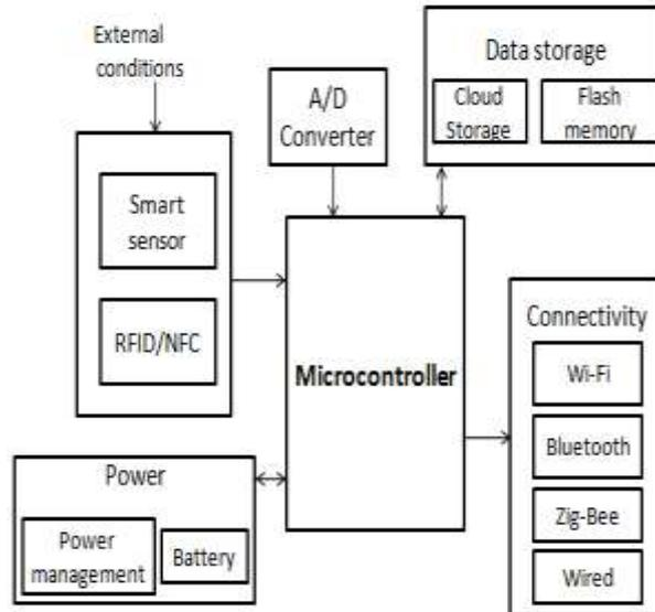
Fig 1: Sensor Node Architecture
