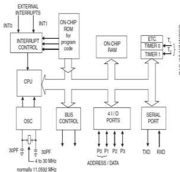
Fig 2: Basic Architecture of Microcontroller 8051
