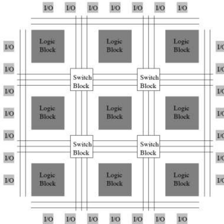
Fig 3 Structure of FPGA
