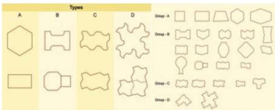
Fig. 1: Different Shapes of Paving Blocks
