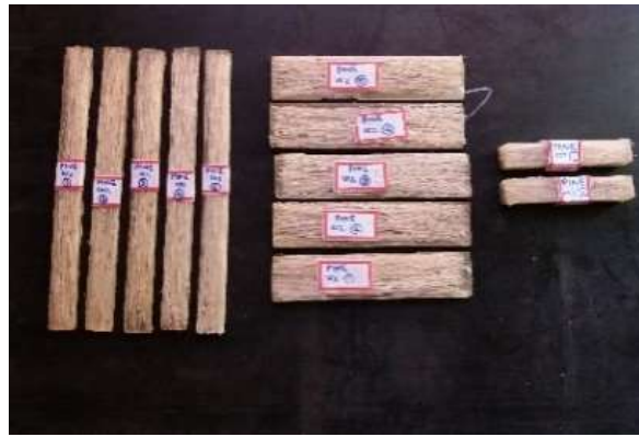
Fig. 3: Specimens of Jute-Hemp Fiber-Polyester Resin Hybrid Composite for Tensile, flexural and Impact
