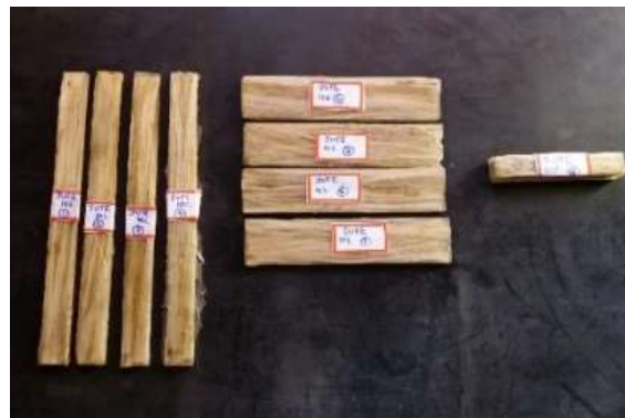
Fig. 1: Specimens of Jute – Polyester- Resin for Tensile, Flexural and Impact
