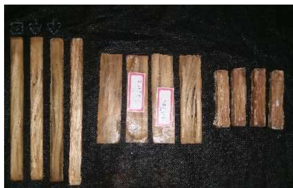
Fig. 2; Specimens Hemp Fiber – Polyester Resin for Tensile, Flexural and Impact
