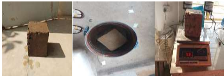
Fig. 3: Water Absorption Test Conducted in Lab
