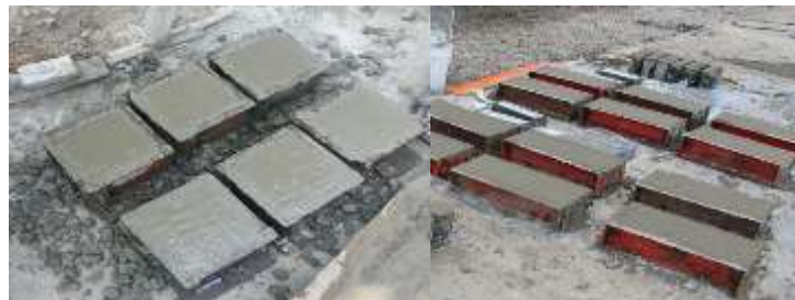
Fig. 1: Casting of Cubes, Beams, and Cylinders
