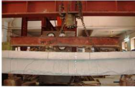
Control Beam after Cracking
