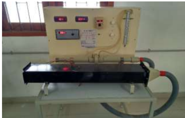
Fig 1 Experimental Setup for Pin Fin Apparatus
