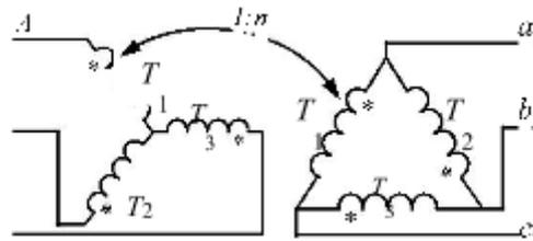
Fig. 8 Wye-delta Connection of the Transformer for Step-down Application
