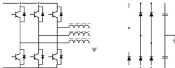
Fig. 6 Three-phase High Power dc/dc Converter
