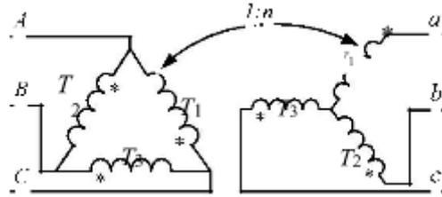
Fig. 7 Delta-wye Connection of the Transformer for Step-up Application
