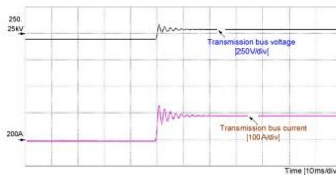
**Fig.12: The Transient Characteristic of HVDC Transmission Bus**
