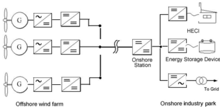
Fig. 3: The Typical Structure of HECI Integrated WPCS
