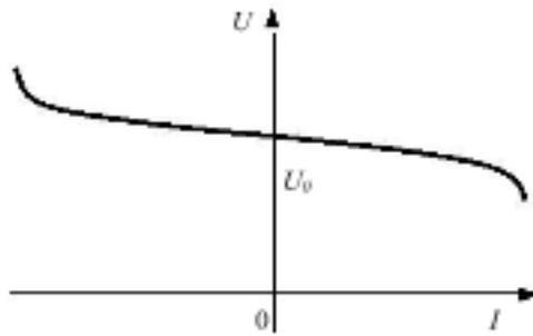
Fig. 5 V-I Characteristic of Battery
