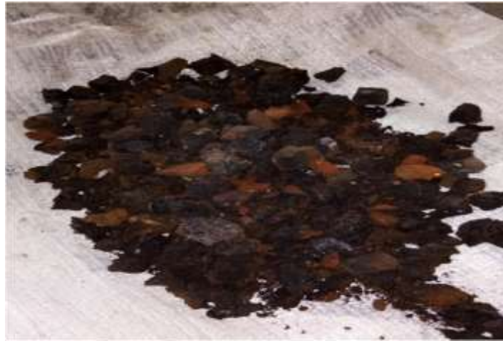
Fig. 1 Over Burnt Bricks
