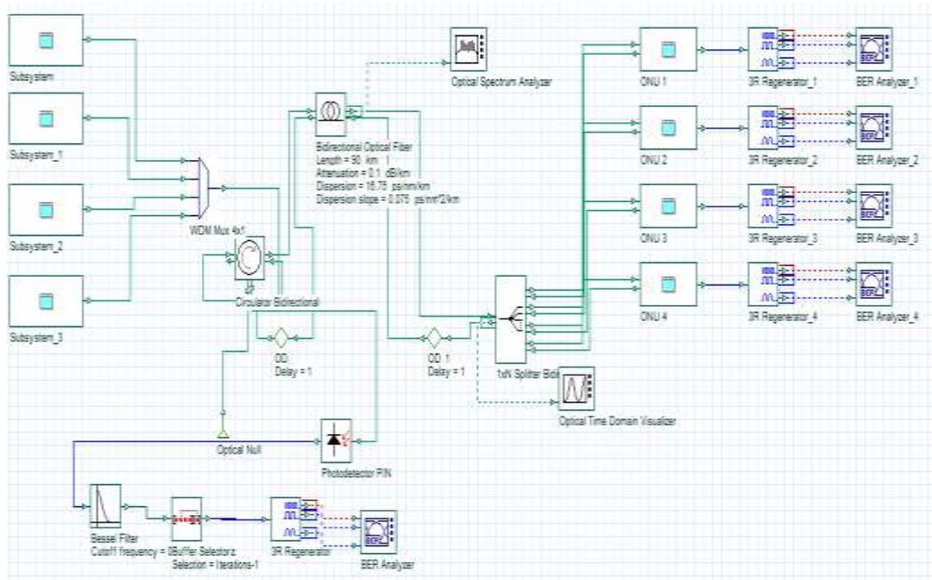
**Figure 2.2 Design of 8 Channel Bidirectional Link**
