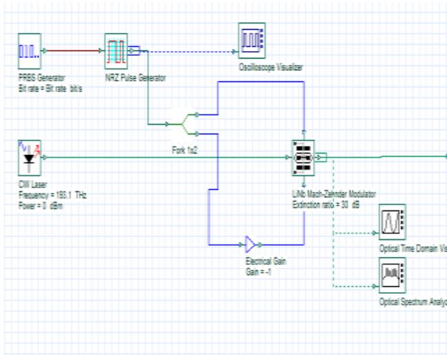
Figure 3.1(a) Design of Subsystem of NRZ Modulator
