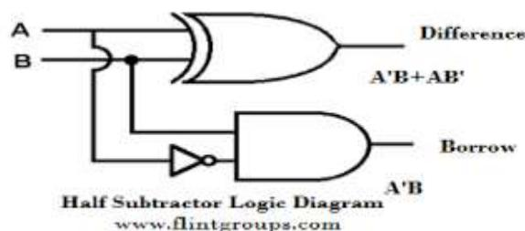
Figure 1.2 logic diagram of half subtractor
