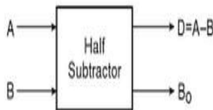
Figure 1.1 logic symbol of half-subtractor
