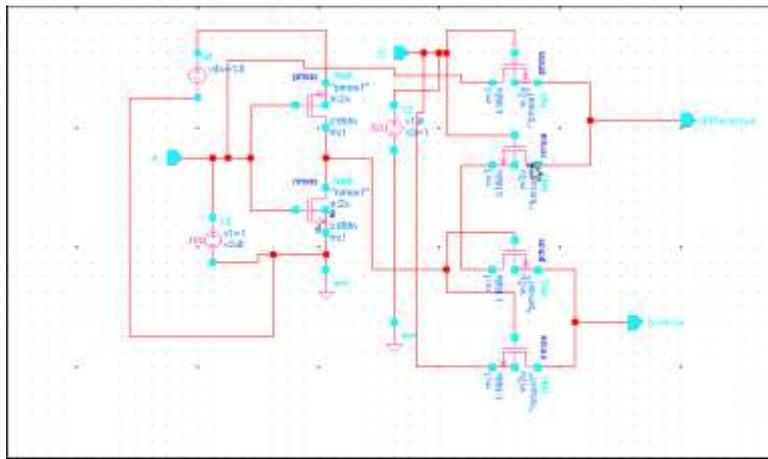
Figure 1.3 Circuit of conventional half-subtractor
