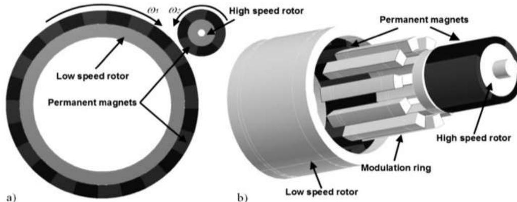
Figure (1). Schematic construction of magnetic gear
