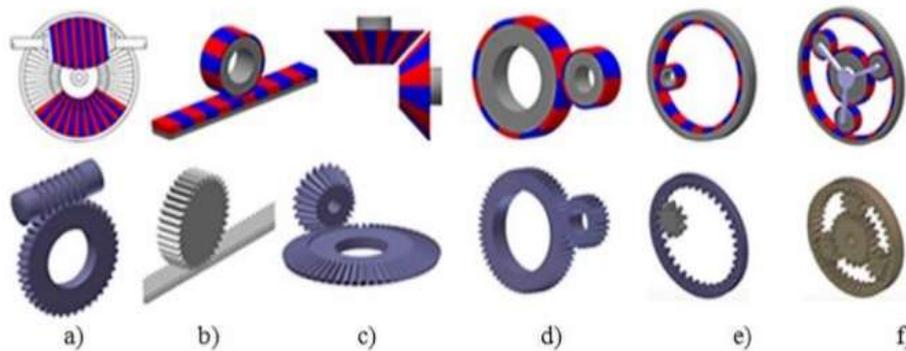
Figure (2): Comparative display between magnetic and mechanical gears.
