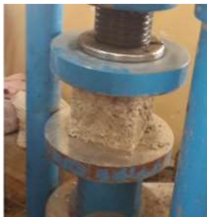
Fig1: Specimen Placed in CTM
