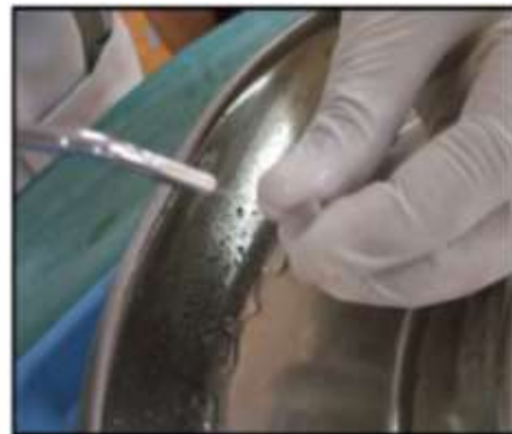
Fig 4: Application of silane coupling agent and drying
