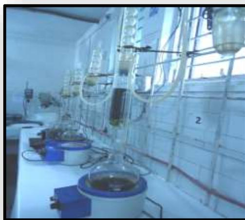
Fig. Showing Soxhlet apparatus
