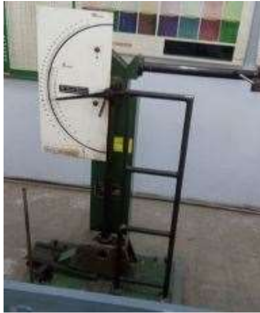
Figure 5. Experimental set up of izod testing of specimens.
