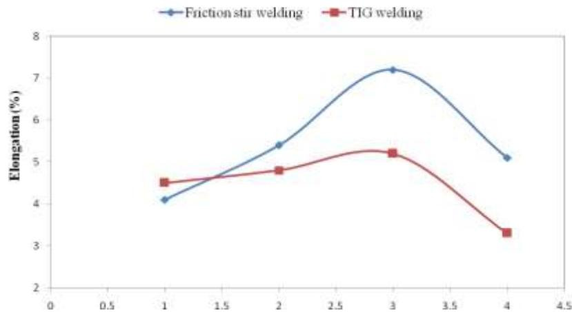
Fig. 4.2: Comparison between Elongation (%) of FSW and TIG Welding
