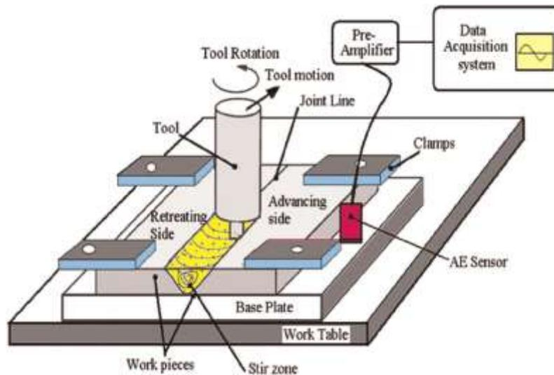
Fig1.1 Schematic Diagram of FSW Process
