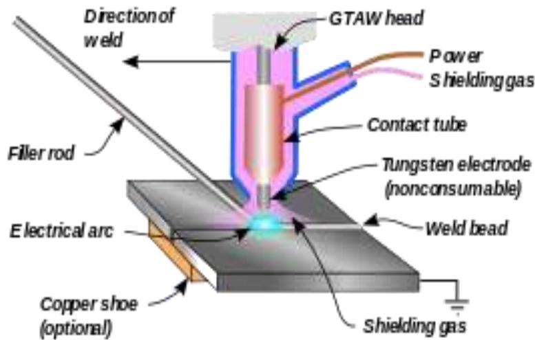
Fig. 1.2 Schematic Working of TIG Welding
