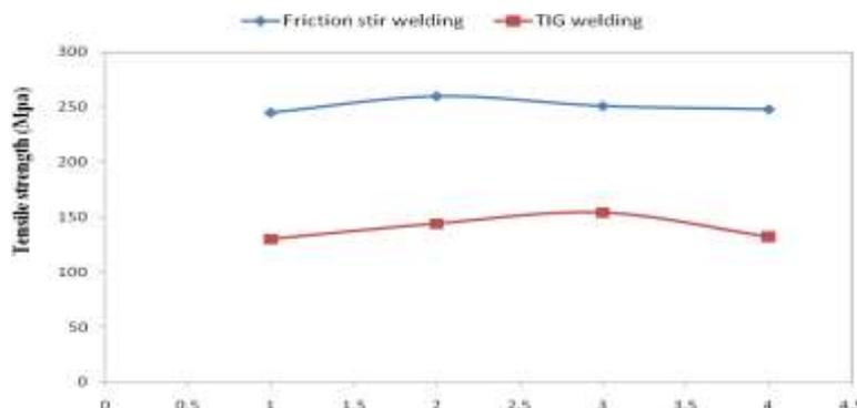
Fig. 4.1: Comparison between Tensile strength of FSW and TIG Welding
