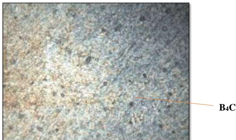
**Fig. 12** Microstructure of Zn-Al alloy reinforced with 3% B<sub>4</sub>C
