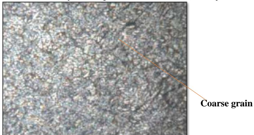
Fig. 10 Microstructure of Zn-Al alloy without reinforcement from the microstructure of Zn-Al alloy [Fig. 12] it is clear that grains which are formed are coarse, this is the reason behind in getting low hardness.
