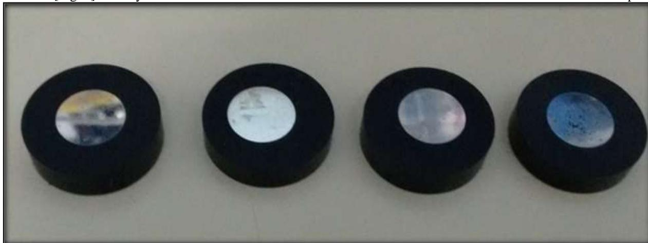
Fig. 6 Samples for studying microstructure
