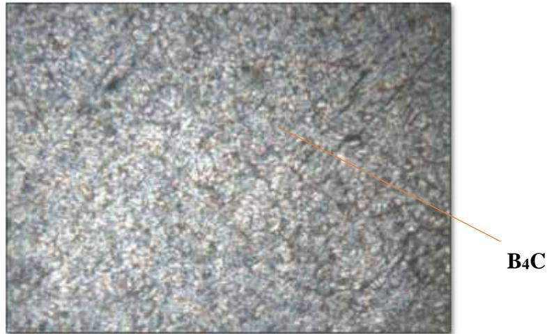
**Fig. 11** Microstructure of Zn-Al alloy reinforced with 1% of B<sub>4</sub>C
