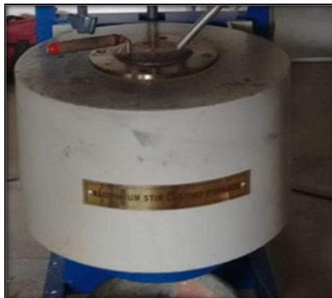
**Fig. 1 Aluminium stir casting furnace**
