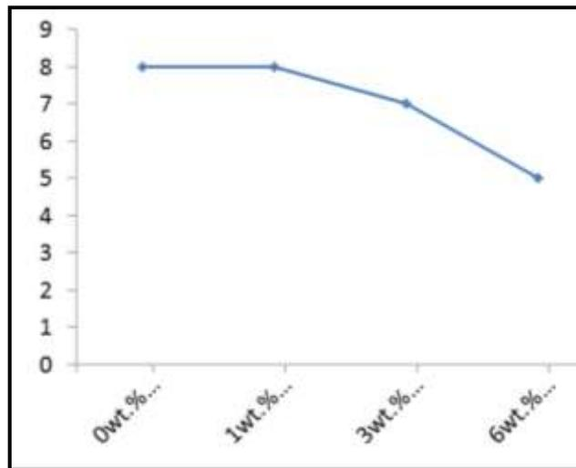
Fig. 9 Graph- Reinforcement Composition vs % elongation
