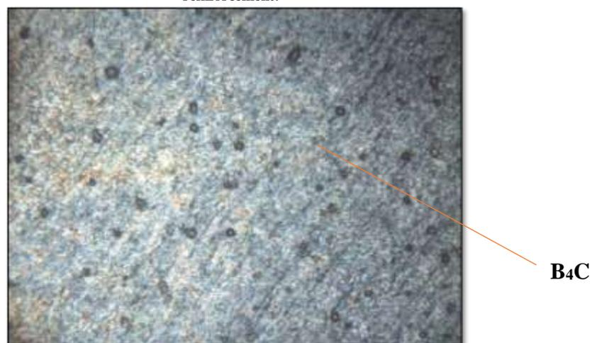
**Fig. 13** Microstructure of Zn-Al alloy reinforced with 6% of B<sub>4</sub>C
