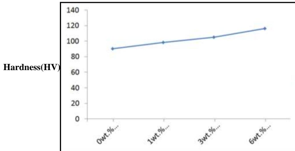
**Fig. 7 Graph-Reinforcement Composition vs Hardness**
