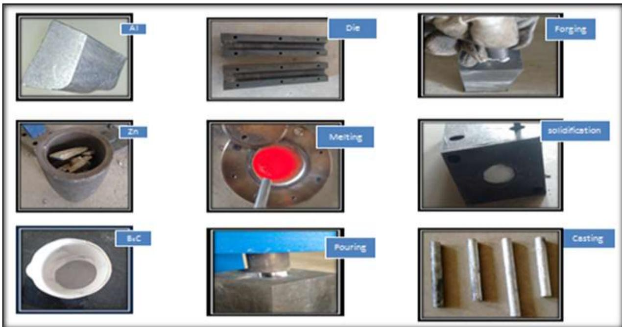
Fig. 3 Stir Casting Process
