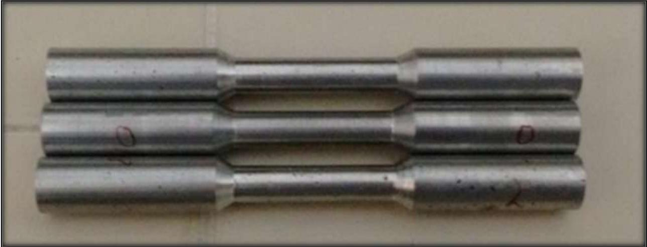
Fig. 4 samples for tensile testing
