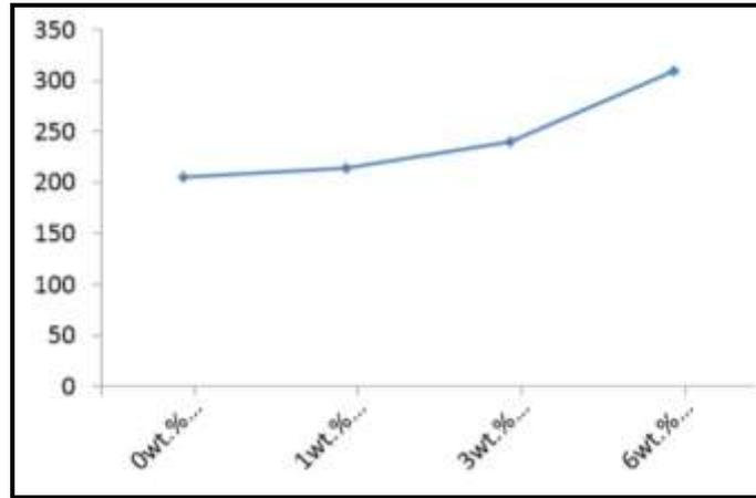
Fig. 8 Graph- Reinforcement Composition vs. Tensile Strength
