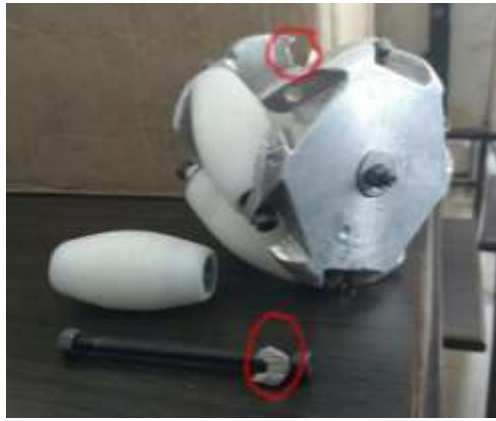
Figure 5: deformation of the wheel after compression
