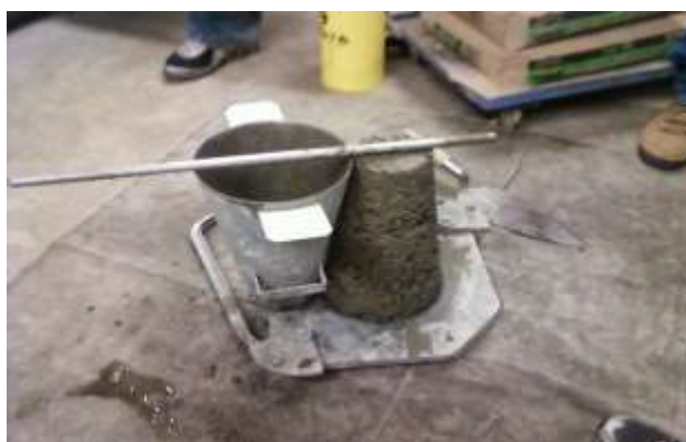
Slump Cone Test
