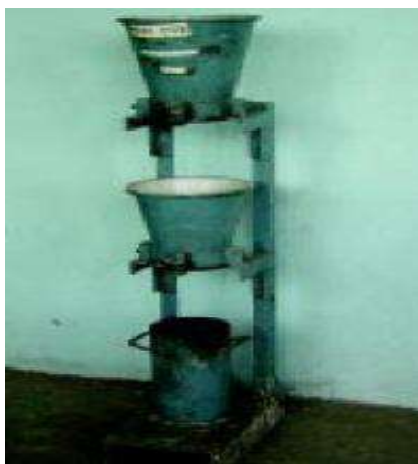
Compaction Factor test
