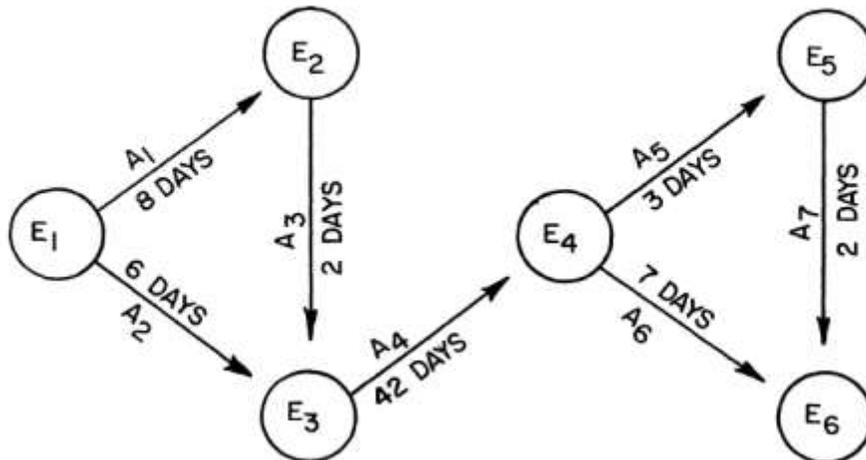
The diagram shows that the longest path which takes the maximum number of days is: E1-E2-E3-E4-E6, in the number of days:  $8+2+42+7=59$  days. The figure below shows the critical path for this example.
