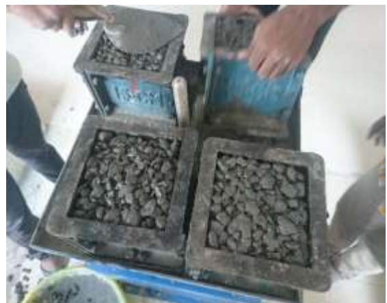
Figure 2: casting of cubes and prism
