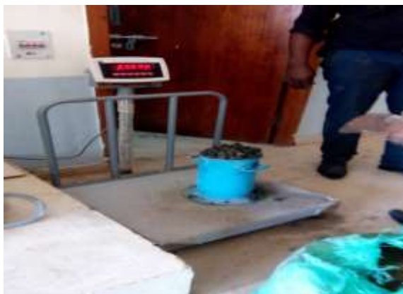
Figure 4: Compaction Factor Test
