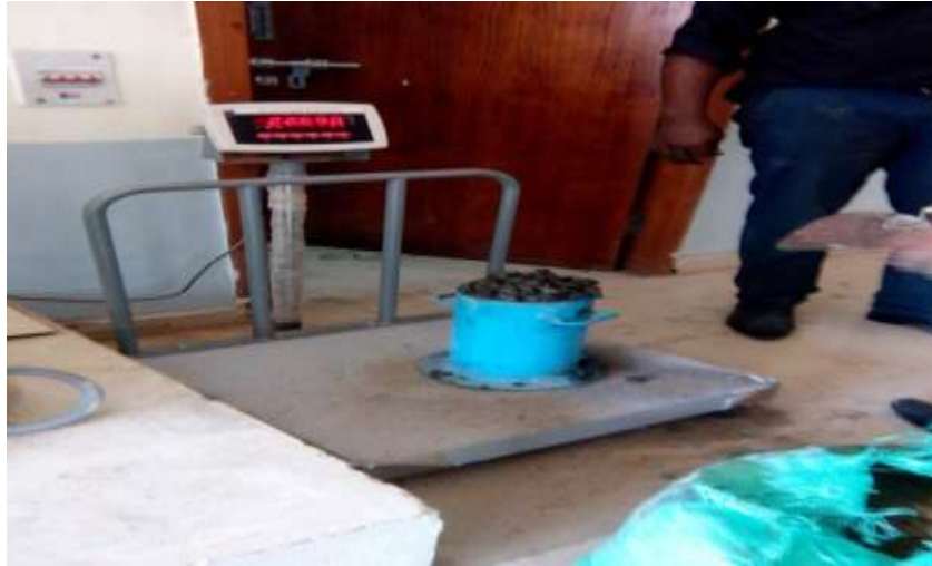
Figure 4: Compaction Factor Test
