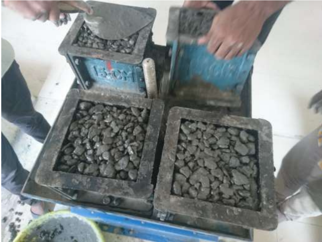
Figure 2: casting of cubes and prism
