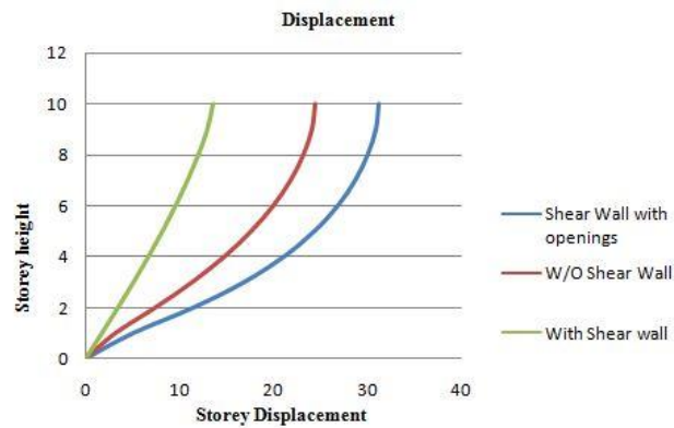
Fig. 4 Comparison for storey displacement between unsymmetrical buildings without shear wall, with shear wall and shear with openings
