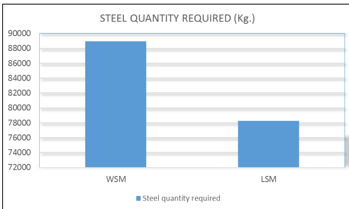
Figure No.5 Comparison Required Steel Quantity
