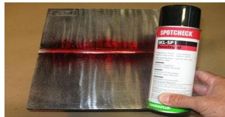
**Remove penetrant.** This usually involves rinsing part, often using an emulsifier to assist with the removal of the excess penetrant. In some applications the penetrant may be wiped from the inspection area
