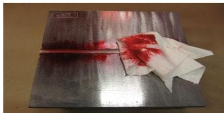
**Apply developer.** A developer is used to draw the trapped penetrant dye out of the defect onto the component surface and also provide a background against which the defect indication will be readily visible. In fluorescent penetrant systems
