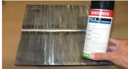
**Penetrant application.** The penetrant dye is applied to the surface of the part for a dwell time which is sufficient to allow the dye to seep into any defects that are present.
