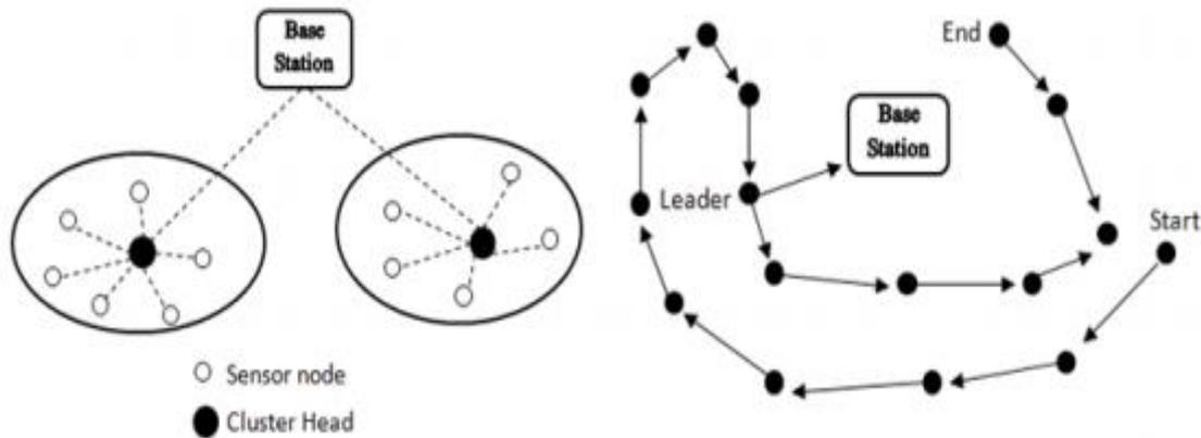
Figure5. Connections between nodes and base station for a) LEACH and b) PEGASIS
