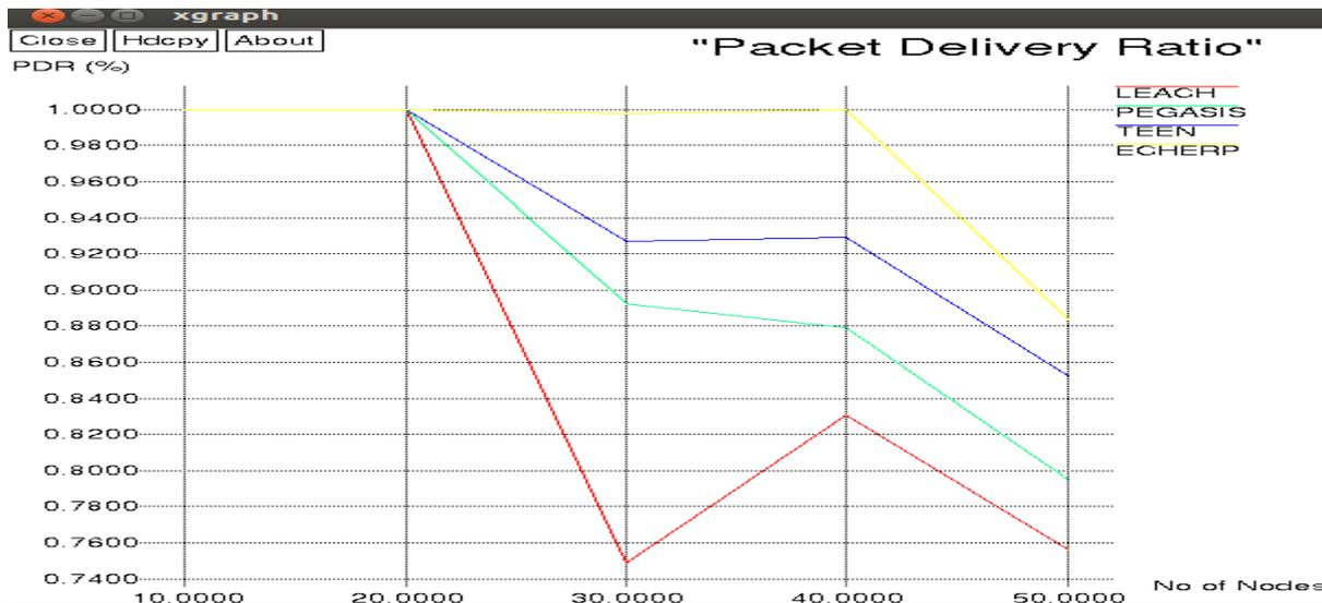
Figure12. Comparison of Packet Delivery Ratio
