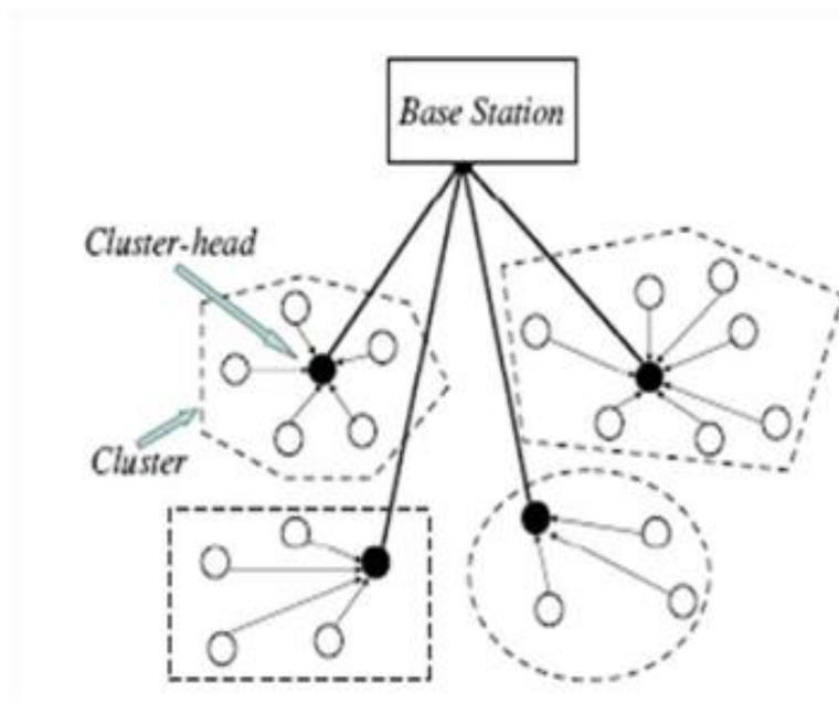
Figure3. Clusters and CHS formation in Hierarchical Routing Protocols
