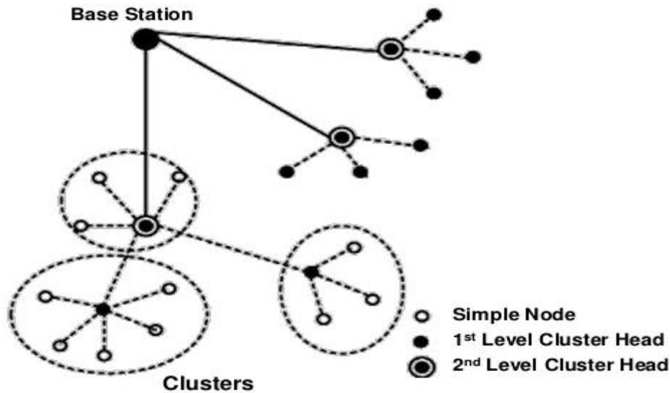
Figure6. Multi level Hierarchical Clustering
