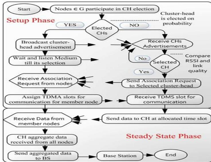
Figure4. Flow chart of LEACH routing protocol
