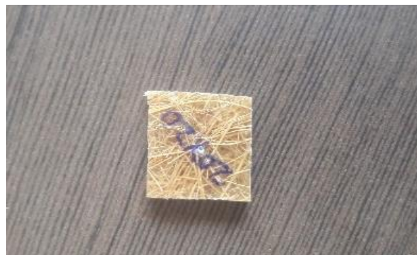
Figure 3.1: Specimen after Hardness Test
