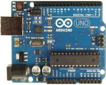
A microcontroller is a small computer on a single integrated circuit. In modern terminology, it is a system on a chip or SOC. A microcontroller contains one or more CPUs (processor cores) along with programmable input/output peripherals Program and memory. memory in the form of Ferroelectric RAM, NOR flash or OTP ROM is also often included on chip, as well as a small amount of RAM.
