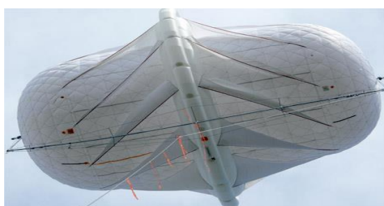
Fig 1: General airborne wind turbine
