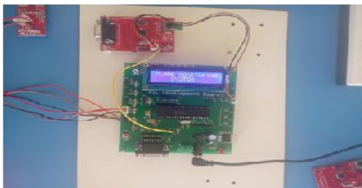
Fig. 10. Implementation of flood monitoring system
