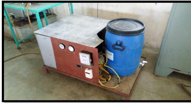
Fig. 6 Air source heat pump setup
