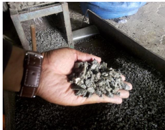
Solid Plastic is then Crushed into grinding machine
