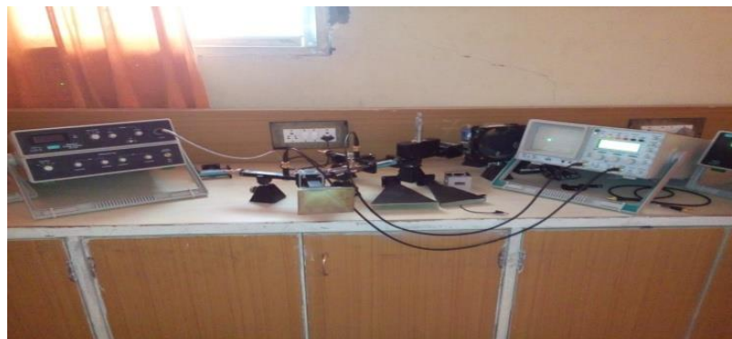
Fig.5: Hardware model for system using microwave test bench (pyramidal horn antenna)
