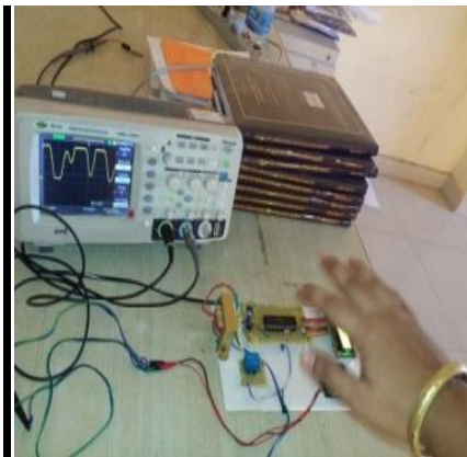
Fig. a: Waveform for Human having motion
