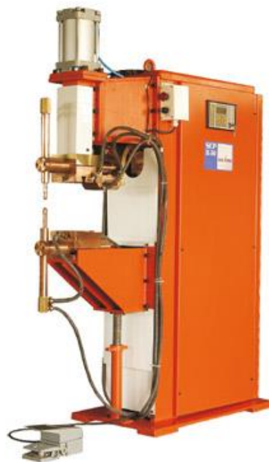
Fig. 3. Resistance welding machine (WELDON INDIA-75)
