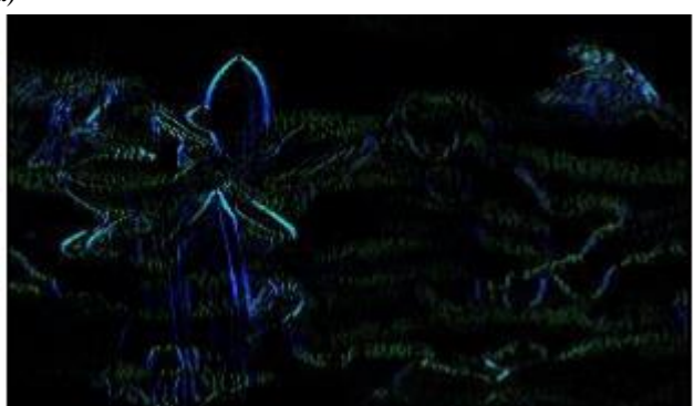
Fig. 5: An example of blur measurement using Edge sharpness analysis (a)Input Image (b)edge magnitude image; Blue- Vertical edge, Green Horizontal edge (c) Sharp edge Image.
