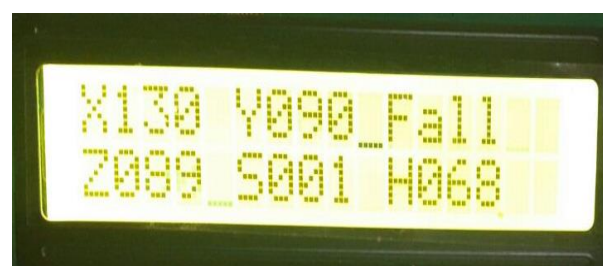
Fig.7 (b) Image showing the LCD display after fall has taken place
