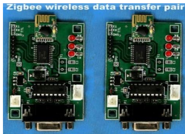
Fig.5 (d) Integrated circuit of Zigbee data transfer pair for transmission and reception
