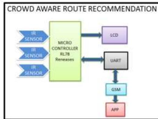
**Figure 4: Architecture Diagram of CARR**
