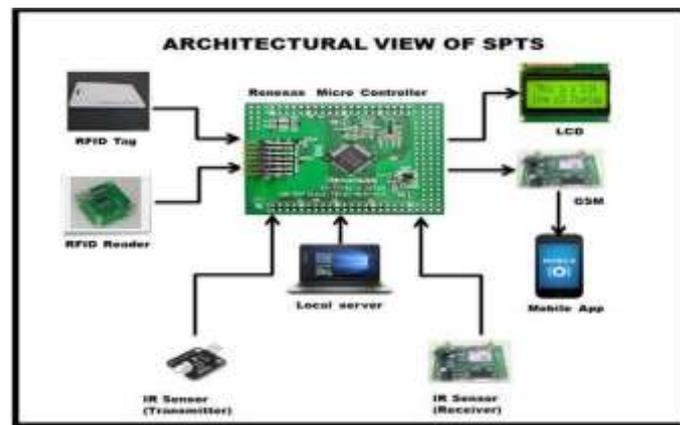
**Figure 1: Architecture Diagram of Smart Public Transport System**
