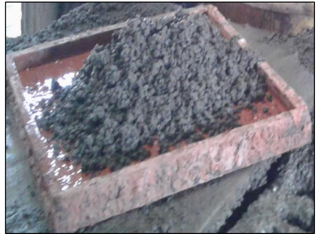
Fig.2.10.Vibration of mould with bottom layer
