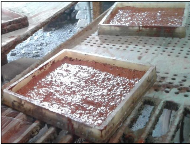
Fig.2.9.Vibration of mould with top layer
