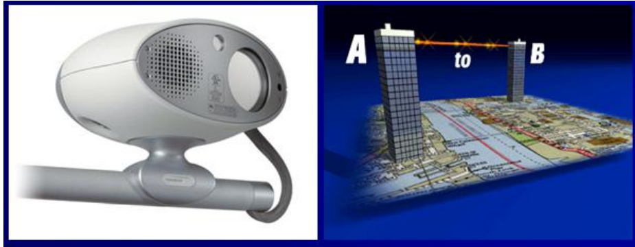
Figure 2 FSO communication between Merrill Lynch Brokerage and Wall Street in New York following the terrorist attack that destroyed normal fiber optic link
