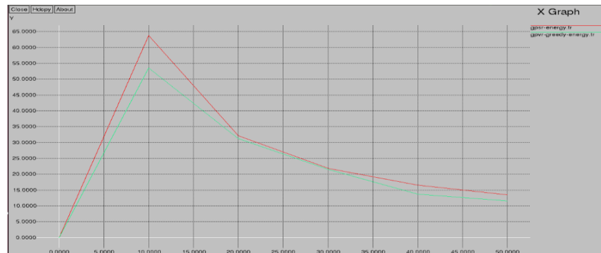
Figure 12 Comparison of GPSR & GPVR protocol in the term of Energy using 10 to 50 Nodes
