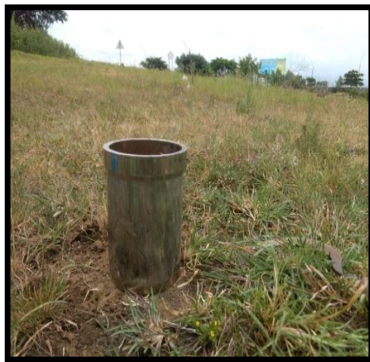
Fig. 5 (a) & (b) - Field density by Core Cutter Method.
