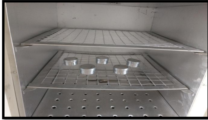
Fig 4 (a) & (b)-Water content by oven drying method.
