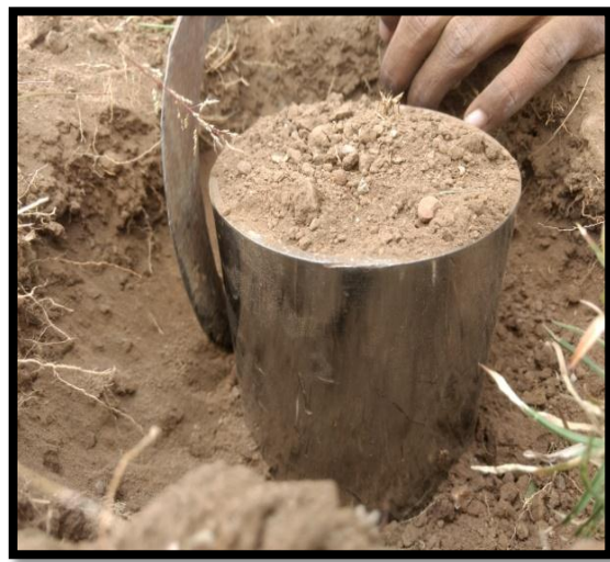
Fig. 5 (a) & (b) - Field density by Core Cutter Method.
