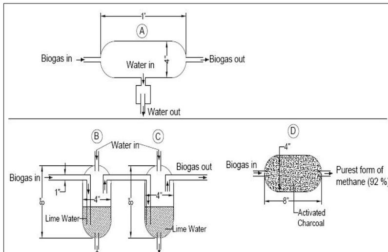
Fig 2 Design of Purification of Biogas
