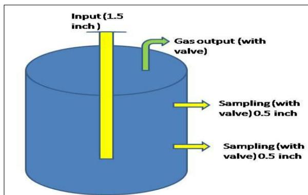
Fig. 6 Layout of experimental setup 3
