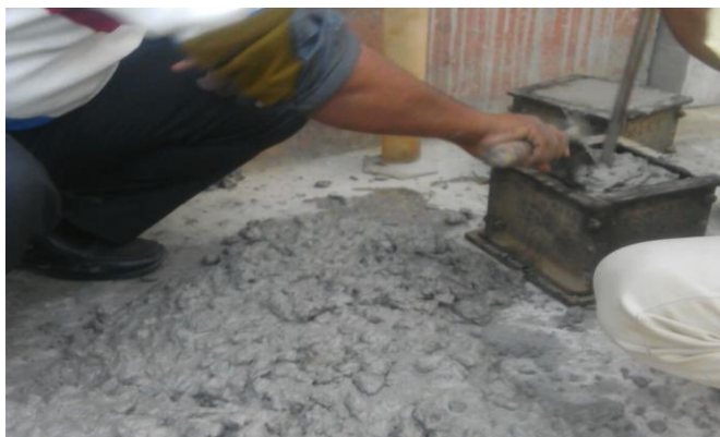
Figure 1: Concrete mix and cube filling
