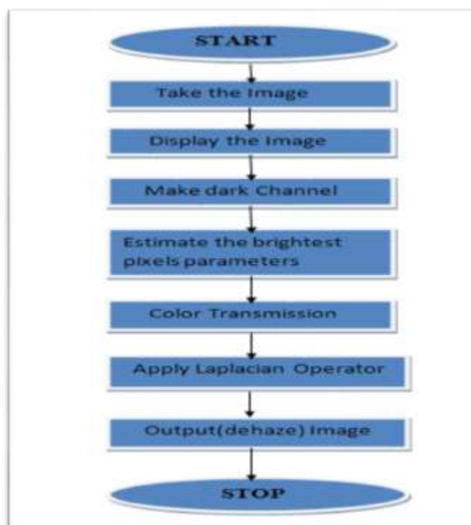
FIG.3 Flowchart for Fog removal algorithm
