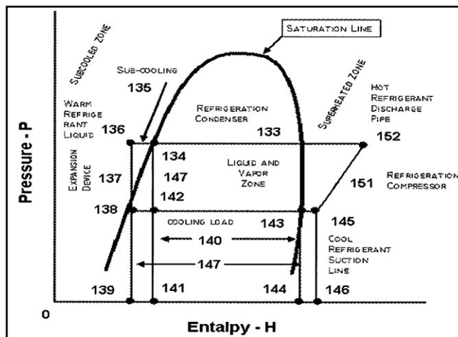
Fig 1.3-the effect of sub-cooling the liquid
