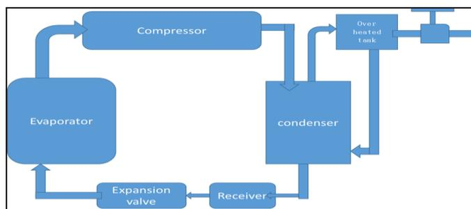
Figure 3.1 Vapour Compression Refrigeration Cycle
