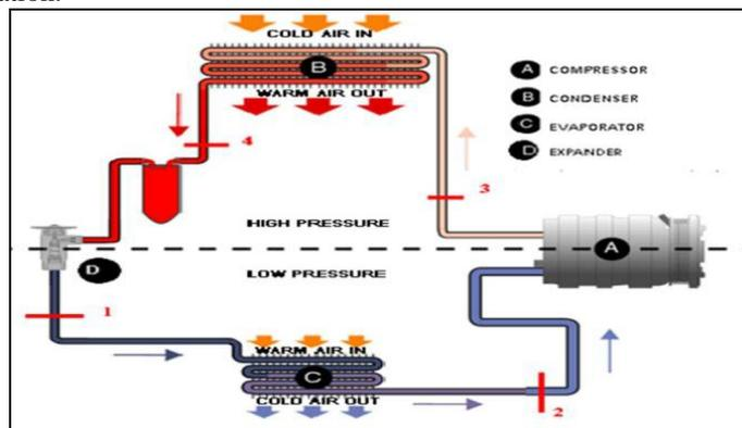
Fig-1.1 Vapour compression system
